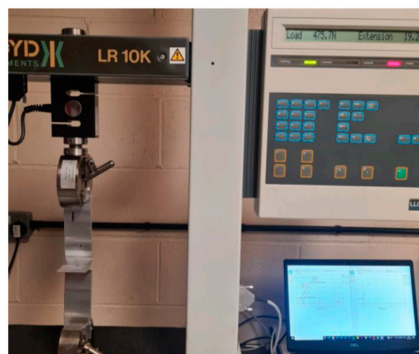
Figure 8. A Lloyd LR10K tensile tester used to conduct pull tests.
