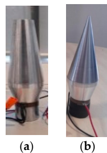
Figure 7. The 20 kHz HPUT used during the laser welding. Transducer configurations: (a) a large tip horn and (b) a small tip horn.
